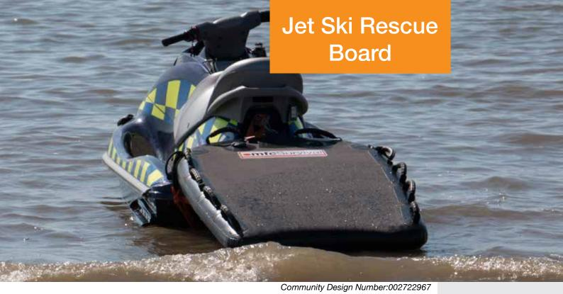
The Jet Ski Rescue Board is an inflatable board that is attached to the back of jet ski by a towing 'D' ring and two shock cord 'D' rings which are located at the front .
